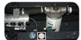
RÉSERVOIR D'HUILE HYDRAULIQUE INCORPORÉ AU CHÂSSIS
